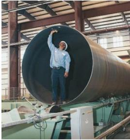
AMERICAN SpiralWeld manufactures steel pipe in diameters up to 144 inches.
